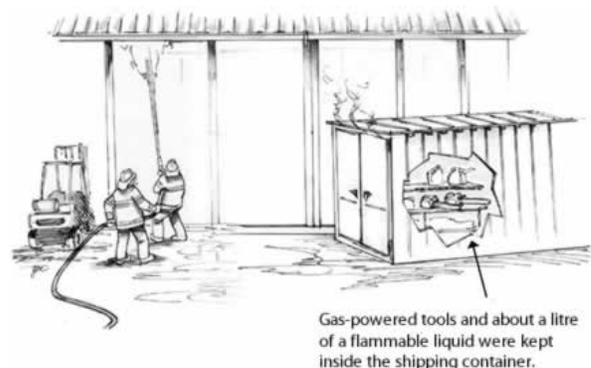
*A shipping container that held small amounts of flammable liquids was exposed to extreme heat when the building next to it caught fire. The evidence indicates that the flammable liquids vaporized and exploded, blowing off the container's doors.*
