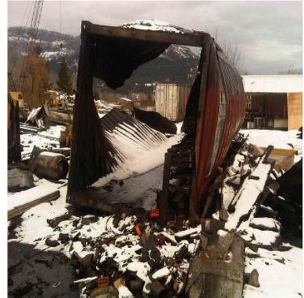
In Saanich in April 2013 a leaking barbecue tank stored in a shipping container exploded and destroyed the shipping container. In this incident, the parts of the container landed 274m [300 yards] away and the walls were flattened. Luckily, no one was seriously injured in this incident.
